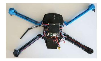
Turn IRIS over, and remove the bottom shell. You should be able to pull the arms partially away from the body of IRIS.
