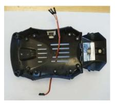
Before you attach the ESC to the bottom shell, you'll need to arrange the cables so they will be situated properly to connect to Pixhawk.
