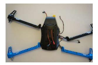
Thread the red-and-black two-wire cable with the red JST connector through the slots in the bottom shell.
