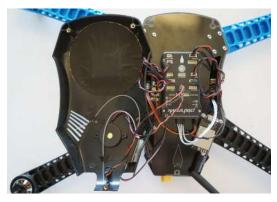
Lastly, you'll connect the components from the top shell to Pixhawk and reattached the top shell.
