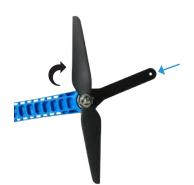
To remove, hold the motor in place with the propeller tool, and spin the propeller in the direction of the unlocking symbol.
