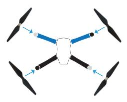
Each propeller has locking and unlocking direction symbols. To attach, spin the propeller in the direction of the locking symbol. The propellers will automatically tighten onto the motors when you arm IRIS before takeoff.
