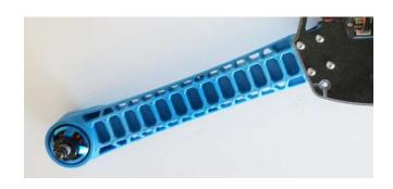
Remove the four screws holding each arm in place.
