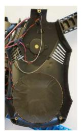
Now add the GPS shield to the top plate. Remove the adhesive backing, and stick the shield to the inside of the top shell around the GPS module so that it is completely covered and the cables are arranged as neatly as possible.
