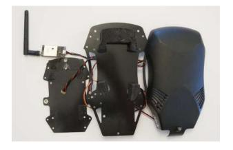
Once the smaller, bottom plate is detached from the foam. Turn it over and remove the four screws attaching the ESC to the plate. You should now be able to remove the ESC and the arms entirely from the plate.
