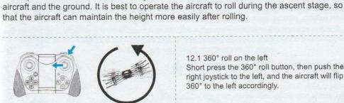
The aircraft can achieve 360-degree flight by the following joystick operation. In order to
