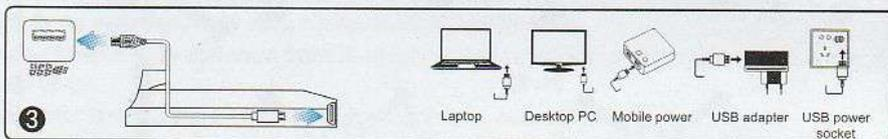
6.3 Charging: Insert the USB interface of the USB charging line into the USB port of the computer (or use the power adapter with output of 5V  $\overline{=}$  2A), and connect the plug at the other end of the USB charging line to the battery socket. The USB red light of the aircraft will go out when charging. The red light will always be on when the battery is full and the charging is completed.
