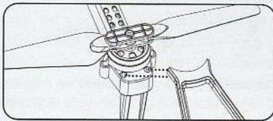
According to the figure, align the protection ring parts with the arm hole to make the connection, confirm the installation is in place before flying to avoid falling during the flight.
