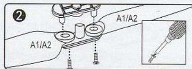
5.2 Loosen the screw, open the two fan blades and the connecting parts, and remove the fan blades for replacement. (When A1/A2 fan blade is broken, replace A1/A2, and so do to B1/B2 fan blade, error in replacement will cause that it can't take off)
