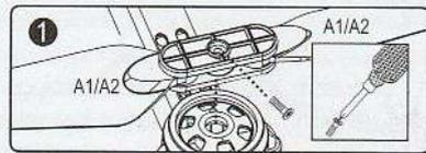
5.1 Unscrew the screw and remove the fan blade.
