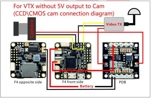
ii).CMOS camera 5V can also be connected to the J17 RAW, but need to short circuit J3 RAW and 5V solder joints
