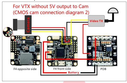
3. Stripes appear when some racing drone up/down throttle, if you do want to fix it, please connect the battery power cord to PDB power input, PDB output 5V to FC 5V (PDB must have sufficient current for 5V output)
