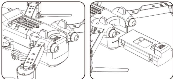
A. Remove the lithium battery from the bottom of the drone.
