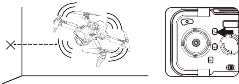
Press the button to turn on the obstacle avoidance mode, and press again to turn off the obstacle avoidance mode.
