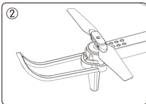
Align the protective frame with the arm and install it (Figure 1), press it until it is in place, and then press the position (Figure 2) up to fasten the protective frame.
