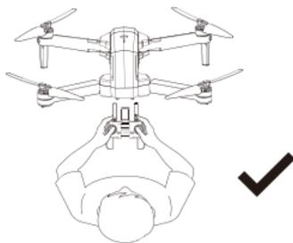
The direction of control when the drone is paired.
