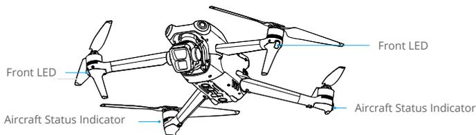
When the aircraft is powered on but the motors are not running, the front LEDs glow solid green.
