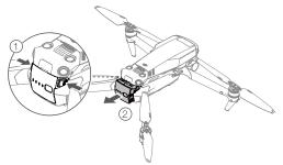
• DO NOT detach the battery when the aircraft is powering on.
