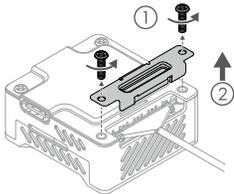
2. Use an appropriate tool (tweezers) to disconnect the cable from the air unit and then remove the camera module with the coaxial cable.
