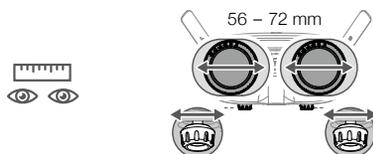
7. Slowly rotate the knobs to adjust the diopter. The supported adjustment range is from -8.0 D to +2.0 D.
