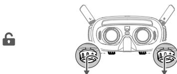
6. Toggle the knobs left and right to adjust the distance between the lenses until the images are properly aligned.
