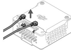
3. Prepare the new antenna. Align the plugs with the antenna connectors on the air unit, press the plugs down to make sure they are securely connected.
