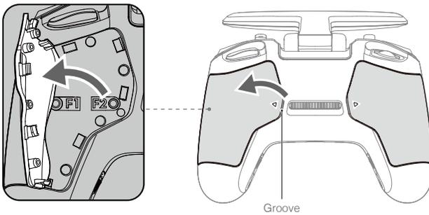
2. Use an H1.5 hex key to adjust the resistance of the stick and recenter the stick vertically. The control resistance increases when the F1 screw is tightened, and the control resistance decreases when the F1 screw is loosened. The recentering is disabled when the F2 screw is tightened, and the recentering is enabled when the F2 screw is loosened.
