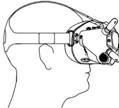
4. Turn the Interpupillary Distance (IPD) slider to adjust the distance between the lenses until the images are properly aligned.
