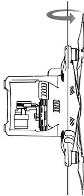
**⚠** If the Aircraft Status Indicator blinks red and yellow after the calibration procedure, move your aircraft to a different location and try again.
