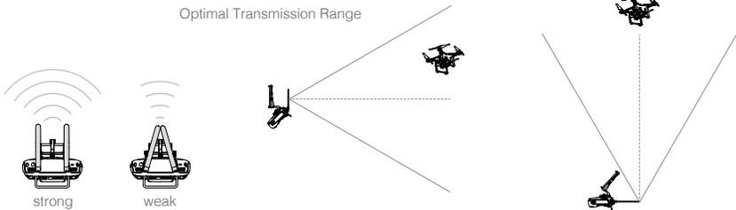
Ensure that the aircraft is flying within the optimal transmission zone. To achieve the best transmission performance, maintain the appropriate relationship between the operator and the aircraft.
