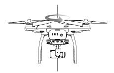
Hold the aircraft vertically, with nose pointing downward, and rotate it 360 degrees around the center axis. Recalibrate the compass if the Aircraft Status Indicator glows solid red.
