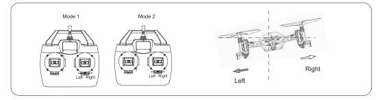
Move the aileron trim right if the UFO flies leftward during taking off; otherwise move it left.
