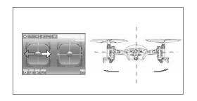
(4) Rotate control: When moving the RUDD control ball left, the UFO accordingly rotate left(CCW); When moving the RUDD control ball right, the UFO accordingly rotate right(CW).
