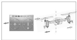
(2) Aileron stick control (left and right): When moving the phone to the left, the UFO will fly to the left; when moving the phone to the right, the UFO will fly to the right (The control ball won't scroll in mode 1 and mode 4 while in mode 2 and mode 3, the ball will scroll.)
