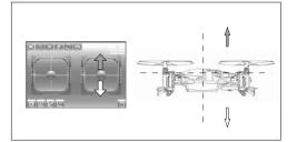
(1) Throttle stick control: Press and hold the throttle control ball and then pushed up, the motor rotates, the higher it push, the faster the motor will rotate(fly higher); The motor will slow down when push down, the lower it push, slower the motor rotates.
