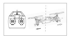
4. When moving elevator stick up or down, the UFO according flies forward or backward.
