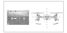
(4) Rotate control: When moving the RUDD control ball left, the UFO accordingly rotate left(CCW); When moving the RUDD control ball right, the UFO accordingly rotate right(CW).
