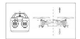
2. When moving the throttle stick up or down, the UFO accordingly flies up or down.
