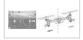
(2) Aileron stick control (left and right): When moving the AILE control ball left, the UFO accordingly flies left; When moving the AILE control ball right, the UFO accordingly flies right.
