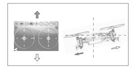
(3) Elevator stick control(forward and backward): When moving the phone to the front, the UFO will fly forward; when moving the phone to the back, the UFO will be backward. (The control ball won't scroll in mode 1 and mode 4 while in mode 2 and mode 3, the ball will scroll.)
