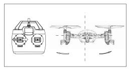
3. When moving the rudder stick left or right, the head of UFO accordingly flies left or right.
