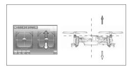
(1) Throttle stick control: Press and hold the throttle control ball and then pushed up, the motor rotates, the higher it push, the faster the motor will rotate(fly higher); The motor will slow down when push down, the lower it push, slower the motor rotates.
