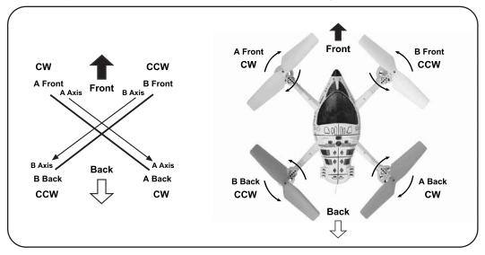
2. After connecting the power of the QR W100S, please check the propellers rotation direction, A front/ back propellers rotate CW, B front/ back propellers rotate CCW.
