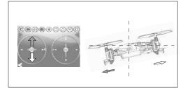
(3) Elevator stick control(forward and backward): When moving the ELEV control ball up, the UFO accordingly flies forward; When moving the ELEV control ball down, the UFO accordingly flies backward.
