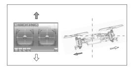
(3) Elevator stick control(forward and backward): When moving the phone to the front, the UFO will fly forward; when moving the phone to the back, the UFO will be backward( For Iphone/ iPad, the controlled ball can't scroll in Mode 1 and Mode 4 mode, but can scroll in Mode 2 and Mode 3 mode).
