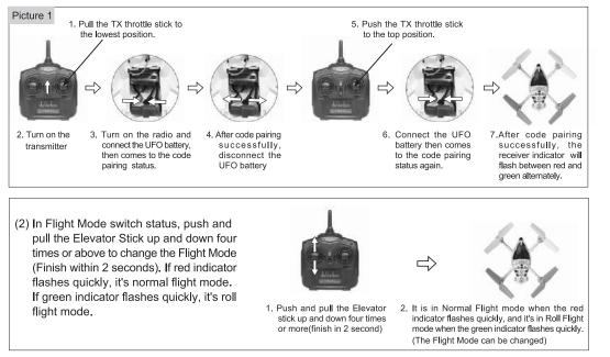
(3) After choose the Flight Mode, pull the throttle stick at the lowest position, then flight available.
