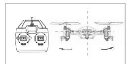
3. When moving the rudder stick left or right, the head of UFO accordingly flies left or right.
