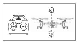
2. When moving the elevator stick up or down, the UFO accordingly rolls forward or backward.
