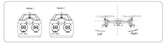
Move the rudder trim right if the head of UFO flies leftward during taking off; otherwise move the rudder trim left.
