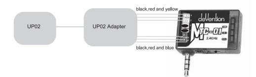
(4) Control Program IC upgrade by RF: Plug the line binded with black,red and yellow into the upgrade channel 3, Plug the line binded with black,red and blue into the upgrade channel 4.
