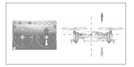
(1) Throttle stick control: Press and hold the throttle control ball and then pushed up, the motor rotates, the higher it push, the faster the motor will rotate(fly higher); The motor will slow down when push down, the lower it push, slower the motor rotates.
