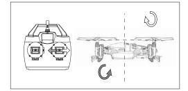
1. When moving the aileron stick left or right, the UFO accordingly rolls left or right.
