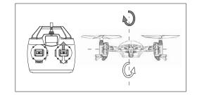
2. When moving the elevator stick up or down, the UFO accordingly rolls forward or backward.
