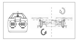
1. When moving the aileron stick left or right, the UFO accordingly rolls left or right.
