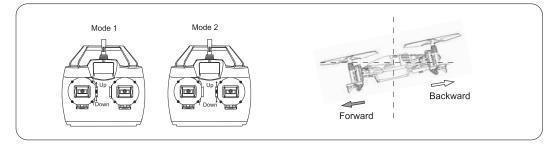
Move the elevator trim down if the UFO flies forward during taking off; otherwise move it up.
