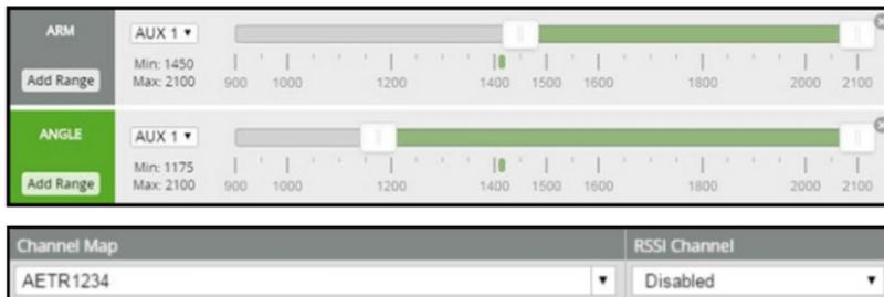
3.Turn on the transmitter and then power on for the QX70, Toggle the switch and the green LED on the flight controller will get be solid, this indicate the motor was armed, enjoy the flight now but be careful !
