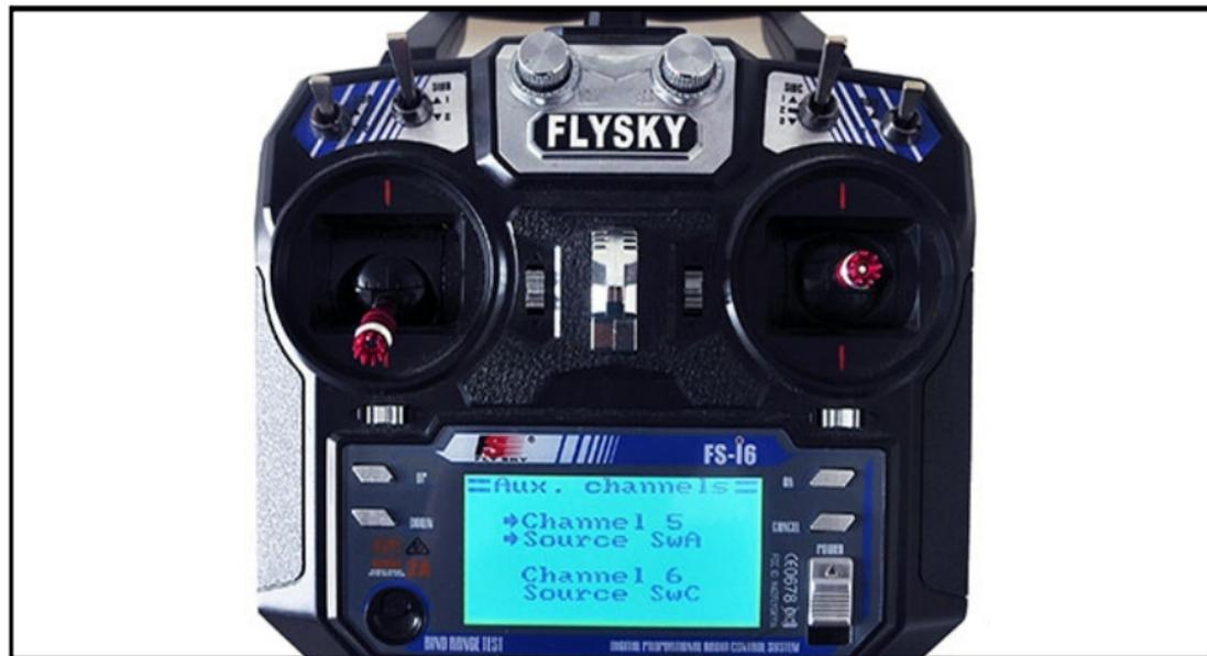
2.The Turbine QX70 was set AUX1(CH5) to ARM/DISARM the motor before shipping ,and you can also customize it with Cleanflight or Betaflight Configurator. The default receiver Channel map for Flysky Version is AETR1234, please ensure your transmitter is matched with it, otherwise it can't be armed.
