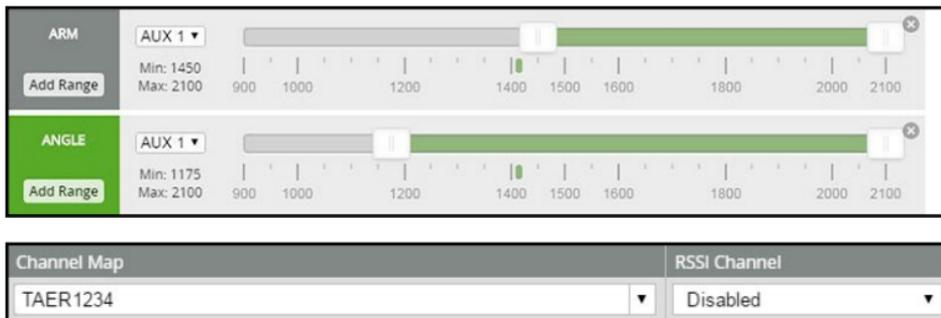
3.Turn on the transmitter and set a switch for CH5 to ARM/DISARM the motor, some transmitter like SPECKTRUM DX6/DX6I, the default CH5 is GEAR Switch.
