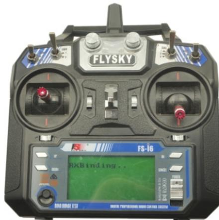
2.Turn on the transmitter while holding the bind button
