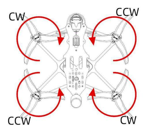
**Note:** If the propeller orientation is incorrect, it will directly affect the Babyhawk O3's ability to fly and be controlled properly. Please carefully inspect and verify the propeller orientation. Regularly check the tightness of the screws to ensure they remain secure during flight. Exercise caution and ensure safety when installing or removing propellers!
