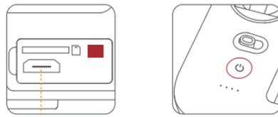
⚠ This 5 pin port is only for updating firmware, but X8 SE Drone is auto equipped with auto update function. So there is no need to use this 5 pin port.
