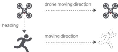
In Lock mode, the drone will hover at a place if flight speed is 0, following the target 360°. The user can also adjust flight speed, and the drone will fly around the target at a certain distance.
