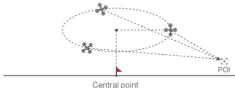
If sticks are moved in flight, the flight altitude or radius will be changed. Taking Mode 2 as example:
