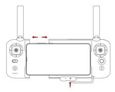
⚠ Note: The cable slot is reserved on the right side of the RC.
