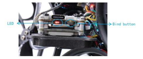
3. The transmitter indicator light changes from blue to green, and the AirUnit indicator light changes from red to green, the bind is successful.
