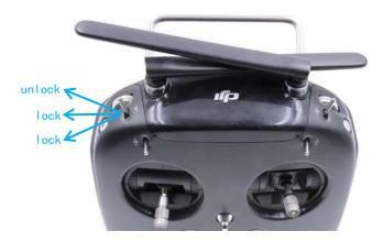
3. When landing, when the height drops to about 30cm from the ground, it can be locked to complete the landing
