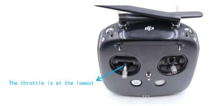
2. When the lock switch is set to the bottom gear, the motor turns. First gear up motor locked
