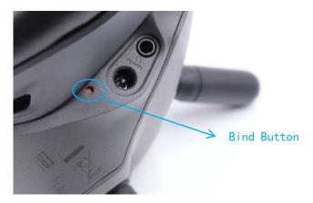
2. Press the bind button at the AirUnit, and the indicator light at the AirUnit changes from green to red, which is the bind state.
