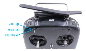
The three modes can be switched in flight or locked. The operation of self stable mode is relatively simple, so it is suggested that the first choice of self stable mode is for novices.
