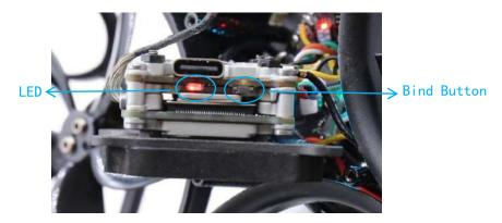
3. The AirUnit indicator light changes from red light to green light. When you see the picture in the goggle, the bind is successful.
