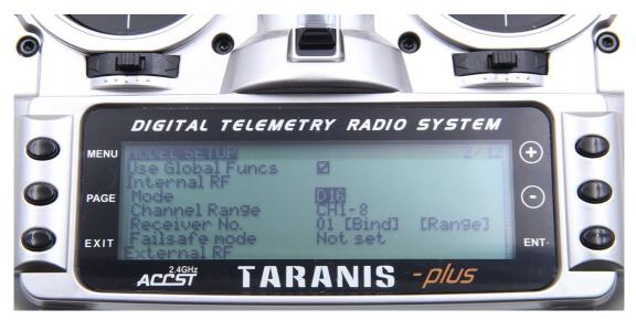
■ 2 : Move the cursor to the "Mode" option , "Mode" option the working mode of XJT can be switched. There are three types of D16, D8, and LR12 respectively. Please select according to your receiver:
