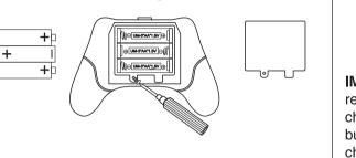
**Step 1** Using the included screwdriver, unscrew the screw from the back of the remote control battery pack and remove the battery lid.
