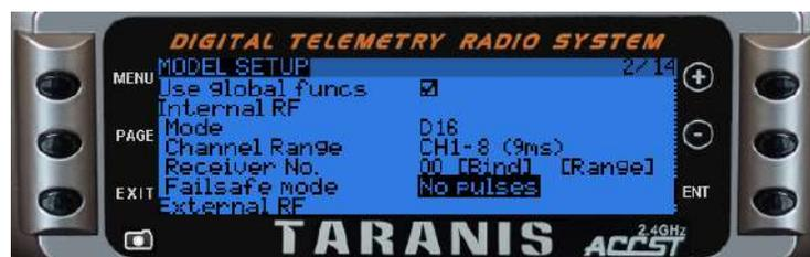
If you have a Taranis with an X-series receiver (bound in D16 mode), you can ensure failsafe is set correctly by choosing "No Pulses" as your failsafe mode in the Model Setup screen. If you have a Taranis with a D-series receiver (D8 mode) this setting has no effect!
