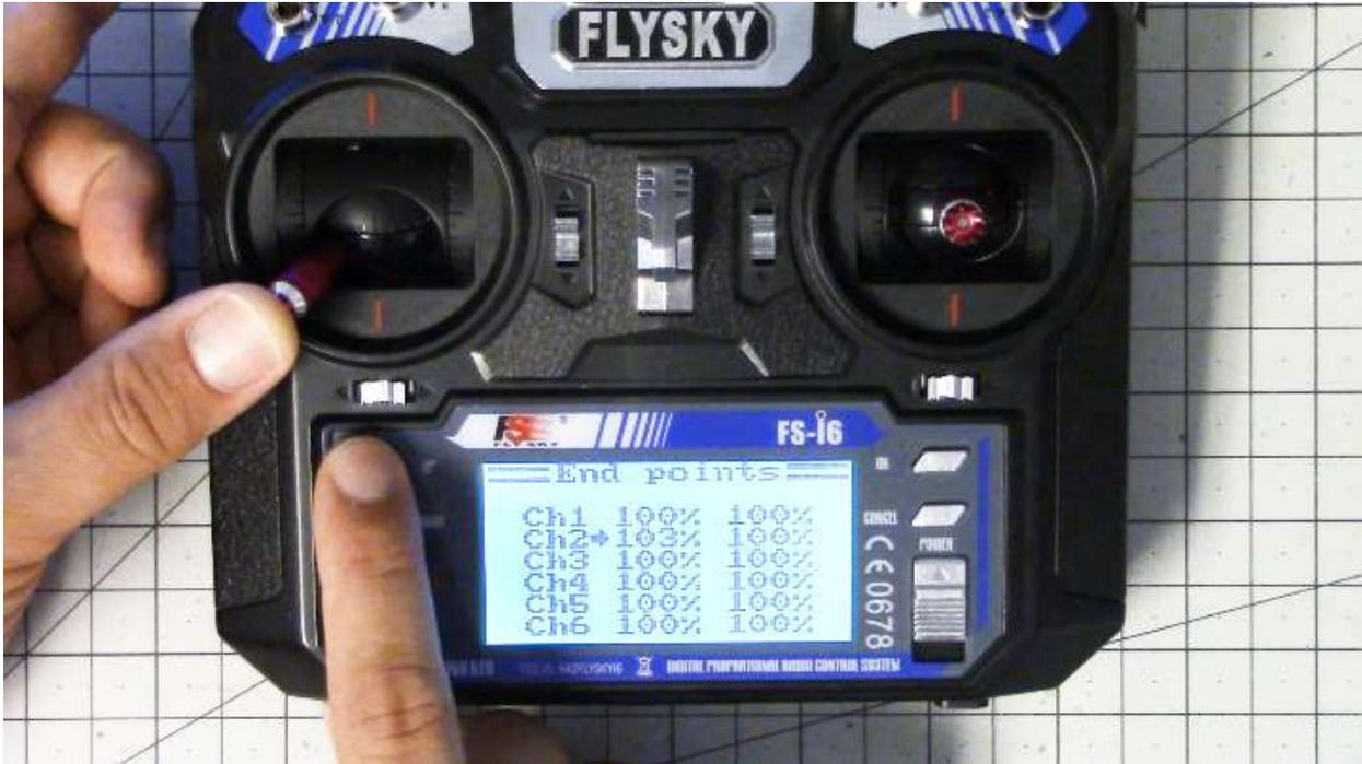
6. In the Endpoints screen, Ok scrolls between channels. Up/Down adjusts the endpoint. You control whether you are adjusting the top or bottom endpoint by raising or lowering the stick for the channel you are adjusting. This can be a little confusing because it's probably not obvious to most people which channel goes with which stick. The default channel order for the FlySky radio and for Betaflight is:
