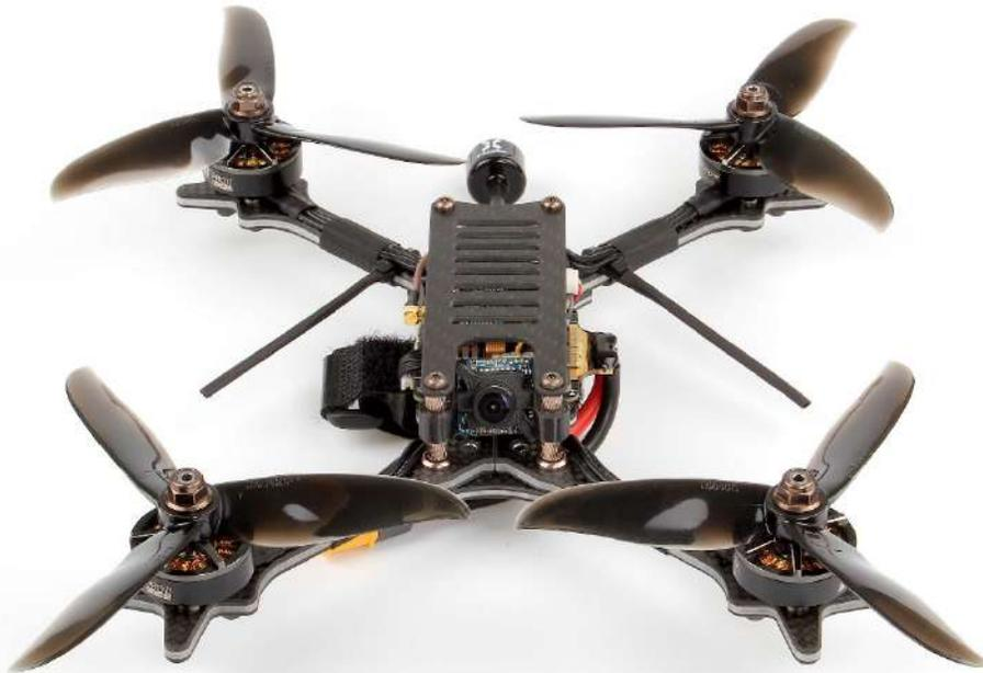
Before shrinking the heat-shrink, tuck or twist any excess length of antenna wire into the body of your KOPIS so that it doesn't get cut by the props or snagged by a branch while flying. Do not kink the antenna wire. Do not cut the antenna wire to shorten it.
