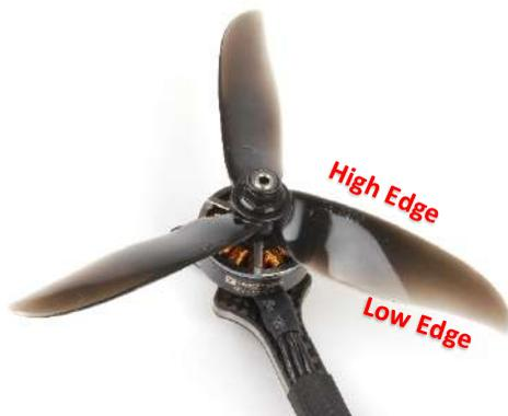
If you look at a prop blade, you will see that there is a *high* edge and a *low* edge. The blade is designed to spin in the direction that the *high* edge is facing.
