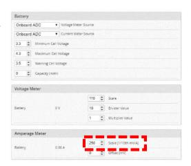
The mAh put back in by the battery will seldom perfectly match the mAh reported by the OSD, but by taking several measurements and averaging the results, you can usually get it reasonably close.
