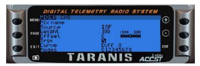
7. Press EXIT to back out to the main menu. Switch SF is now mapped to channel 5, Aux1.
