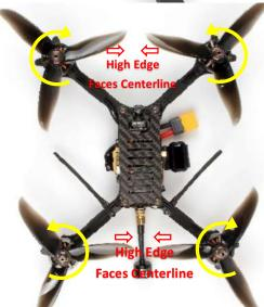
If you look at a prop blade, you will see that there is a *high* edge and a *low* edge. The blade is designed to spin in the direction that the *high* edge is facing.
