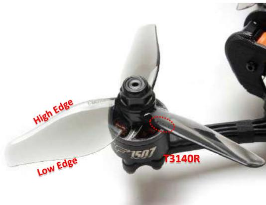
If you look at a prop blade, you will see that there is a *high* edge and a *low* edge. The blade is designed to spin in the direction that the *high* edge is facing.
