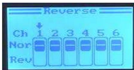
6. Press Ok to cycle through the channels. Press Up or Down to choose whether the channel direction is Normal or Reversed. Reverse the required channels so that the channels move as described above in the Betaflight Receiver Tab.
