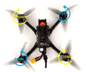
The default motor directions for a Cleanflight or Betaflight quadcopter are shown to the left. Based on this, the correct way to install the props is as shown.
