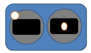
The graphics above show the stick command to bring up the OSD menu. The stick command is: throttle centered, yaw left, pitch forward. The exact stick command therefore depends on which mode your transmitter sticks are in.
