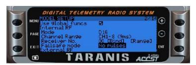
If you have a Taranis with an X-series receiver (bound in D16 mode), you can ensure failsafe is set correctly by choosing "No Pulses" as your failsafe mode in the Model Setup screen. If you have a Taranis with a D-series receiver (D8 mode) this setting has no effect!
