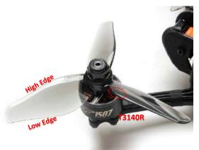
If you look at a prop blade, you will see that there is a *high* edge and a *low* edge. The blade is designed to spin in the direction that the *high* edge is facing.
