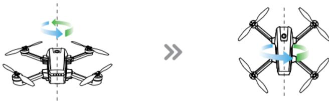
Hold the drone horizontally and rotate the drone in 3 complete circles. When completed the green LED lights will flash.
