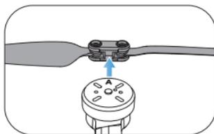
For propeller removal use screwdriver (provided) to rotate counter-clockwise and remove propellers.
