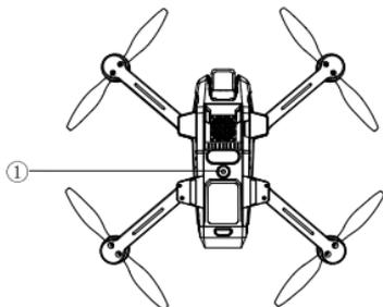
The Optical Flow Positioning System consists of a camera ① module, which acquires the position information of the drone through visual images to ensure precise positioning of the drone.
