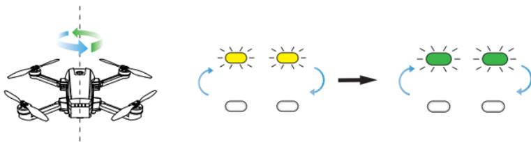
**Step 2:** Hold the drone horizontally and rotate the drone in 3 complete circles. When completed the green lights will flash.
