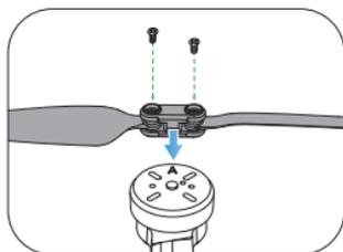
The drone will not fly unless the correct propeller is installed on the correct motor shaft. See illustration above. An “A” or “B” is printed on the back of each propeller. Lock the propeller to the motor shafts with screws rotating each screw clockwise.
