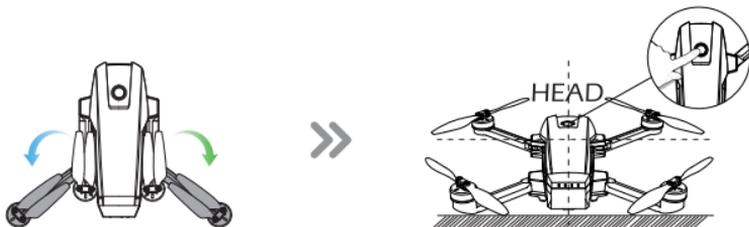
② Short press the Power Switch to turn on the drone, and place it on a level surface with the head forward.
