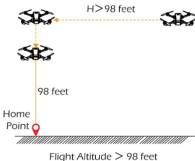
b. When the flight altitude is lower than 98 feet, the drone will elevate automatically to 98 feet high then fly back above the Home Point and exit the First Low Voltage RTH.
