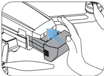
**Installation:** Push the battery into the battery compartment at the rear of the drone. Make sure that you hear a click sound indicating the battery is firmly installed.
