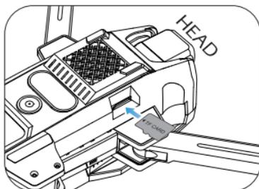
To store your photos and videos, insert the TF card (not included) into the slot as shown above before turning on the drone. The drone supports TF card up to 128 GB.
