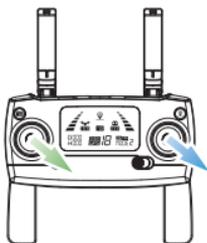
**Step 1:** As shown in the figure above, push both of the joysticks down to the bottom right at the same time to enter the compass calibration.
