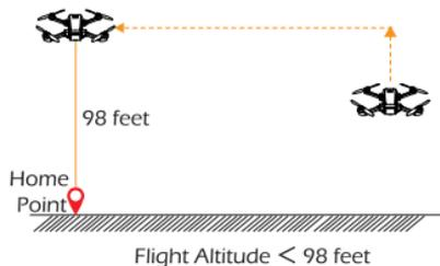
② If the drone's rear lights begin to flash rapidly the “
