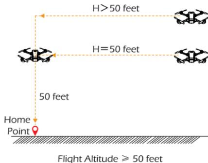
b. When the flight altitude is lower than 50 feet, the drone will elevate automatically to 50 feet high then fly back above the Home Point and descend vertically.
