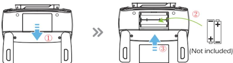
Step 1: Unfold the hand sticks and open the battery cover.
