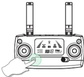
Short press the red button “
