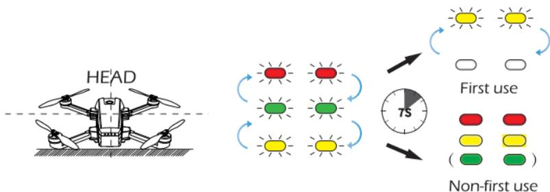
Place the drone on the level surface and it will enter the Initialization Detection. The red, green and yellow lights of the drone will alternate flickering for about **7 seconds** to complete the initial detection. When the transmitter sends out "Di Di", the drone can be divided into two states:
