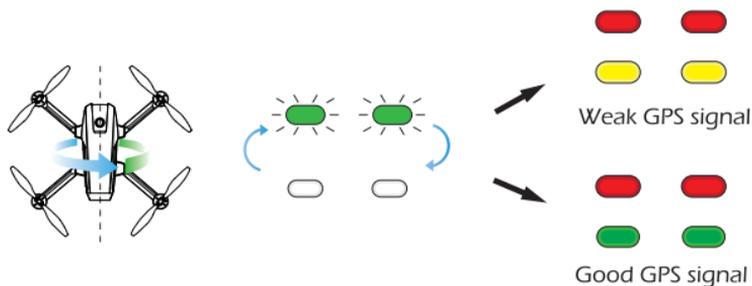
**Step 3:** Hold the drone vertically and rotate the drone in 3 complete circles. When completed the front red lights and rear yellow lights will turn solid and “✖” on the LCD screen changes from slow flash to disappear.
