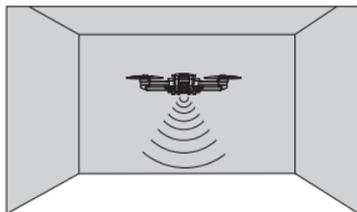
The Optical Flow Positioning System is typically used in indoor environment when GPS is weak or unavailable. It works best when the drone altitude is less than 3 meters.
