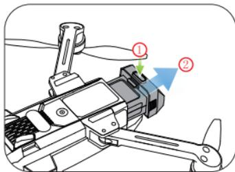
**Removal:** As shown above, press and hold the lock on the back of the battery at the same time while pulling backwards to remove the battery.
