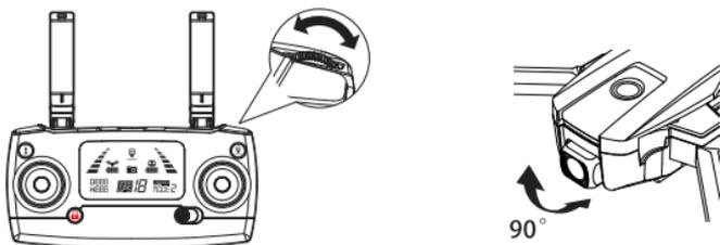
During the flight, you can dial the wheel left / right to tilt the camera up/ down.
