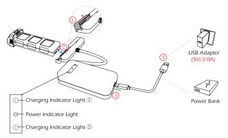
① Connect the Battery, Charger Hub and USB Charging Cable.
