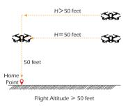
b. When the filght altitude is lower than 50 feet, the drone will elevate automatically to 50 feet high then fly back above the Home Point and desend vertically.
