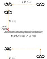
b. When the filght altitude is lower than 98 feet, the drone will elevate automatically to 98 feet high then fly back above the Home Point and exit the First Low Voltage RTH.
