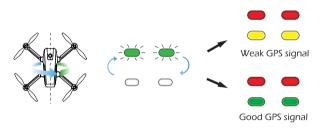
Step 3: Hold the drone vertically and rotate the drone in 3 complete circles. When completed the front red lights and rear yellow lights will turn solid and " \* " on the LCD screen changes from slow flash to disappear.
