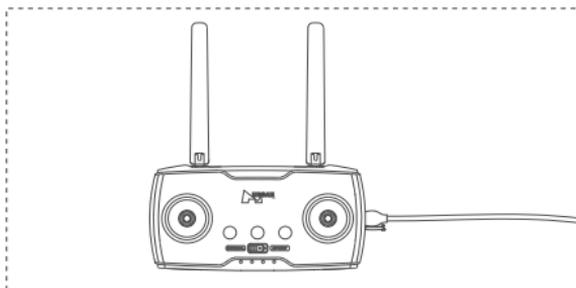
The transmitter charging time is about 2.5 hours. the power indicator of the remote control flashes when charging, and it will solid on after the battery full charged.
