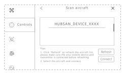
You have to complete the binding process on APP, only when first time using the drone or if replacing the new transmitter.
