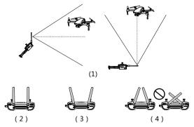
(1) Adjust the angle of the remote control antenna and let it face the flight direction of the aircraft as much as possible.
