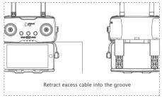
**2.4 Transmitter battery charging** The transmitter uses micro USB cable to charge, as shown in the figure:
