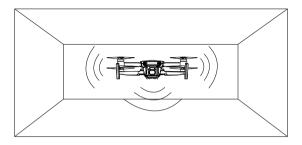
Note: (1). The Vision Systems work best with adequate lighting and clearly marked or textured obstacles. It is not designed to completely replace the pilots controls and judgement, please pay attention to the aircraft and HUBSAN APP tips, and do not rely too much on the Visual systems.
