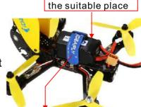
secure the battery with the velcro strap
