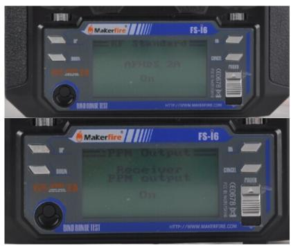
2.Press bind button on RX-2APRO receiver and power the quadcopter at the same time, the orange light will flash quickly when entering bind mode and ready to bind. Press bind button and turn on the remote control at the same time, the quickly flashing light will turn to stay lighted when bind successfully.
