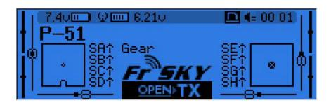
The third shows again the physical switches on the left, and the states of the 32 custom (logic) switches on the right.
