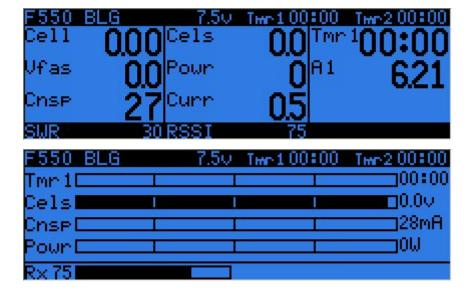
Each field can be one of the various available parameters, of course the corresponding sensors and/or hub must be installed in the model:
