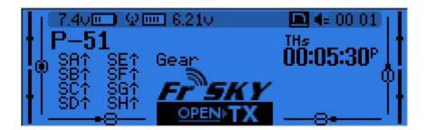
The second shows the gimbal and switches positions, and is handy to check that all the physical controls respond as intended.
