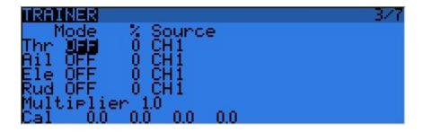
This page allows you to configure the trainer function for "master" use (make sure the Trainer mode in model settings is set to Master). For each of the 4 main functions you will be able to set the mode (OFF, += for Add, := for Replace), ratio and input channel.
