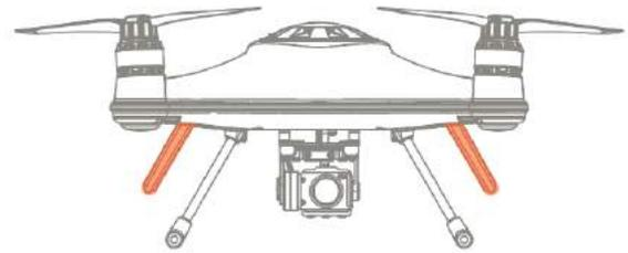
**Antenna oriented downwards:** Improves reception when the aircraft is flying at a high altitude.
