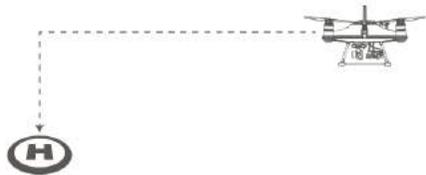
If the aircraft's height is higher than RTH Height (default 20 m), the aircraft will maintain its height and return to the home point.
