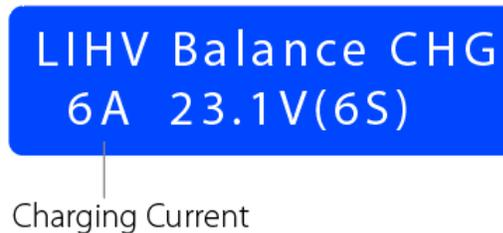
**Lower the charging current to extend battery health. Increase the charging current to increase the charging speed.**
