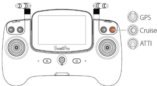
Switch the flight mode toggle to switch the flight mode of the aircraft.
