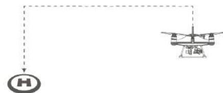
If the aircraft's height is lower than RTH Height (default 20 m), the aircraft will ascend to RTH Height and then return to the home point.
