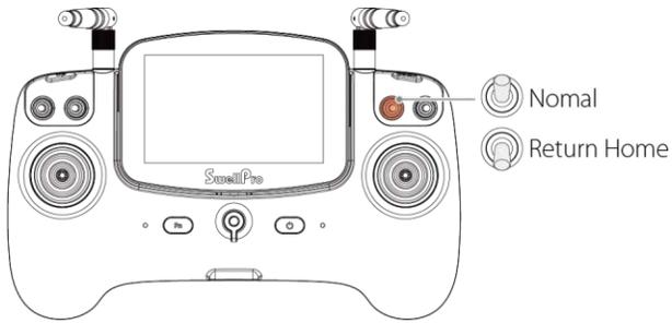
Switch the Return to Home toggle down to “Return Home”. The remote controller would prompt “Return to Home”. The aircraft would start to return to the take-off location.
