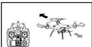
When the aircraft is hovering in the air, in the event that the aircraft is automatically advancing forward or backward, it can be rectified by pressing downwards or upwards the fine-tuning button correspondingly.
