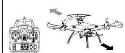
When the right joystick (Turning Rudder) is pushed upwards or downwards, the aircraft will advance forward or backward correspondingly.
