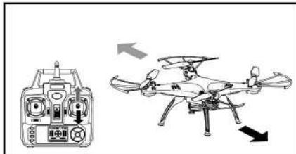
When the right joystick (Turning Rudder) is pushed upwards or downwards, the aircraft will advance forward or backward correspondingly.
