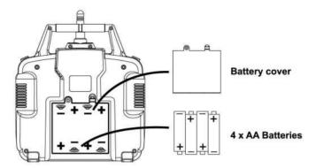
Battery Installation Method: Open up the battery cover at the back of the remote control. Correctly place 4 x AA alkaline batteries in the battery box in strict adherence to the polarity instructions (the batteries are optional).
