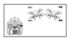
When the right joystick (Turning Rudder) is pushed towards the left or right, the aircraft will fly sideward on the left or right correspondingly.
