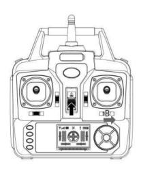
In order to satisfy the different operating habits of the consumers, this remote control is installed with two types of different operating modes, Mode 1 and Mode 2. Upon starting up, press Button B towards the right and switch on the power supply of the remote control simultaneously can toggle between Mode 1 and Mode 2.
