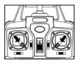
Method 2: Move the left and right joysticks inwards in an internal loop of "8" for 1 second, and the aircraft can be switched off.
