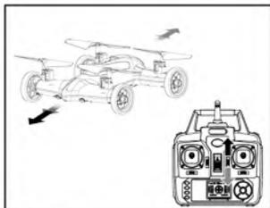
When the quadcopter keeps flying forward / backward, you can correct it by pressing fine-tuning button down / up.
