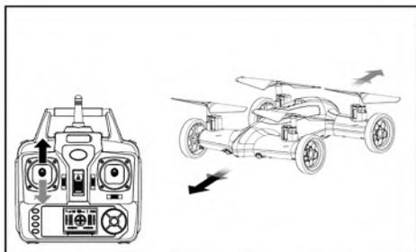
When the aircraft is on the land, operate the left joystick up or down, the aircraft moves forward or backwards accordingly.
