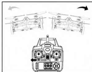
When the quadcopter keeps rotating to left / right, you can correct it by pressing the fine-tuning button right / left.
