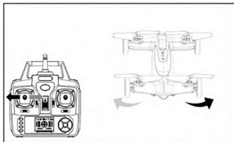
When the aircraft is on the land, operate the left joystick to left or right, the aircraft turns left or right accordingly.
