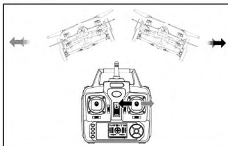
Pull the direction lever left or right, the quadcopter flies to left side or right side.
