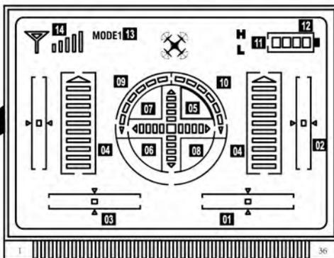
01. Sideward Fine-tuning :Power-on start in the centering.(Be turn Left/Right Fine-tuning in Mode2)
