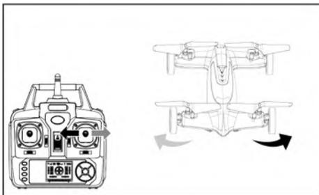
When the aircraft is on the land, operate the right joystick to left or right, the aircraft turns left or right accordingly.
