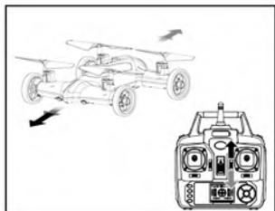
When the quadcopter keeps flying forward / backward, you can correct it by pressing the fine-tuning button down / up.
