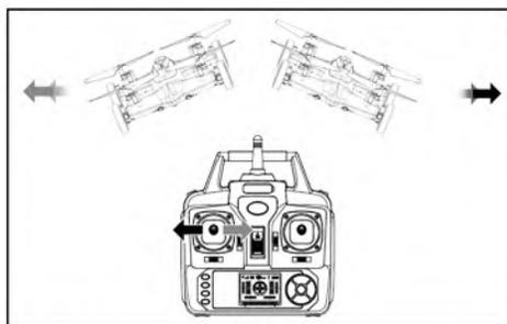
Pull the throttle left or right, the quadcopter flies to left side or right side.
