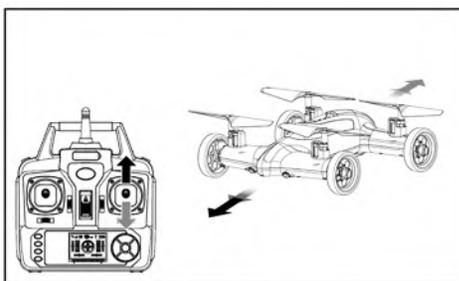
Push the direction lever up or down, the quadcopter flies forward or backward.
