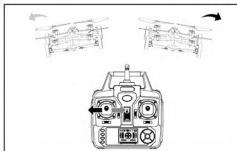
Pull the throttle left or right, the quadcopter turns to left or right.
