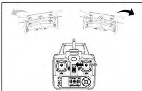
Pull the direction lever left or right, the quadcopter turns to left or right.
