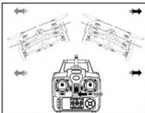
When the quadcopter keeps flying to left / right side, you can correct it by pressing the fine-tuning button right / left.
