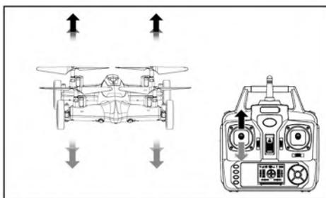
Push the throttle up or down, the quadcopter flies upward or downward.
