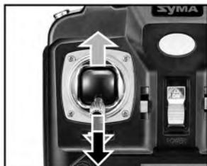
Step 4: Push the throttle lever to the highest position, and then pull it back to the lowest position. There will be one clear sound from the transmitter, this shows that the quadcopter has entered into the pre-fly state.
