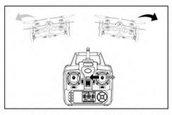
Pull the direction lever left or right, the quadcopter turns to left or right.
