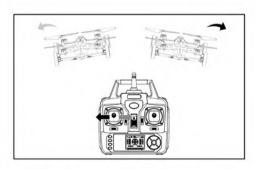
Pull the throttle left or right, the quadcopter turns to left or right.
