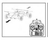
When the quadcopter keepsflying forward / backward, youcan correct it by pressing fine-tuning button down / up.
