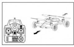
Push the direction lever up or down, the quadcopter flies forward or backward.
