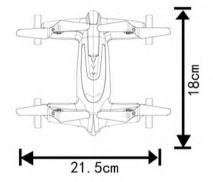
Length of fuselage:180mm Width of fuselage215mm Height of fuselage:65mm Code of main engine: ∮8X4 Battery:3.7V 600mAh
