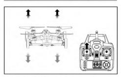
Push the throttle up or down, the quadcopter flies upward or downward.
