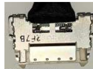
This side of the camera data connector faces the Hadron Camera.
