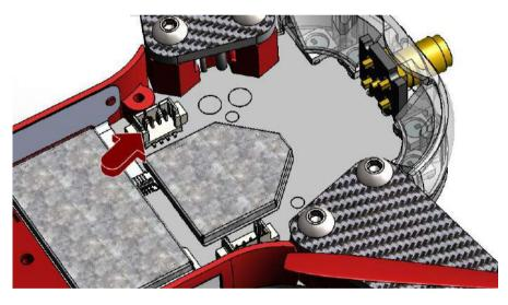
Finally, the receiver antennas may be routed through the two notches in the bottom of the LED diffuser.
