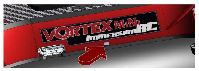
To switch bands, press the button on the LED board for approx. 2 seconds until you hear the first beep, and release. .
