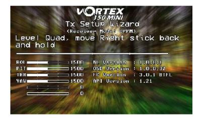
NOTE: To restart the wizard at anytime, power up the quad, press and hold the button on the led board until vortex beeps 2 times (first beep after ~3 seconds, second beep after ~5 seconds). Alternatively you can also enter tx Wizard via OSD menu
