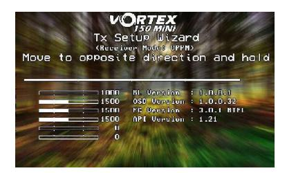
Once the four primary flight controls have been learned, place the quad on a flat and level surface and move the right stick back. This will calibrate the accelerometer.
