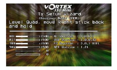
NOTE: To restart the wizard at anytime, power up the quad, press and hold the button on the led board until Vortex beeps 2 times (first beep after ~3 seconds, second beep after ~5 seconds). Alternatively you can also reset the Tx Wizard via OSD menu
