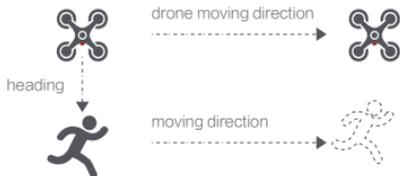
In Lock mode, the drone will hover at a place with its heading trace its target 360-degree if the default speed is 0. The user can also adjust flight speed, and the drone will fly around the target at a certain distance.
