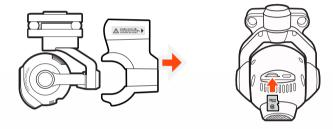
**Step 1)** Remove the cover/lock from the rear of the CGO3 by carefully sliding it backward.
